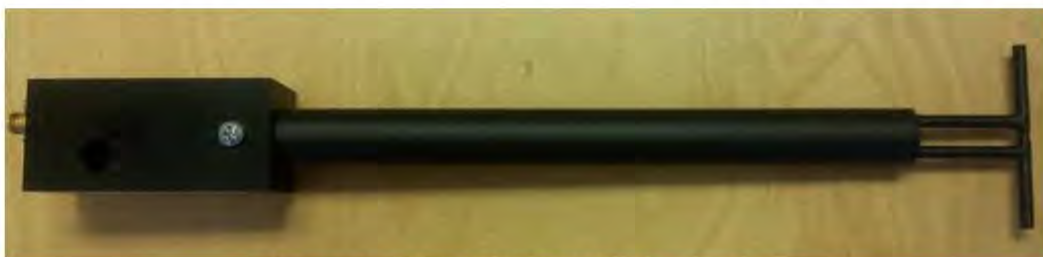
Figure 1 – MVG COMOSAR Validation Dipole
