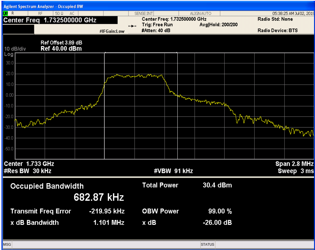
LTE Band4 QPSK BW=3MHz Channel=20175 RB Size=1 Position=#0
