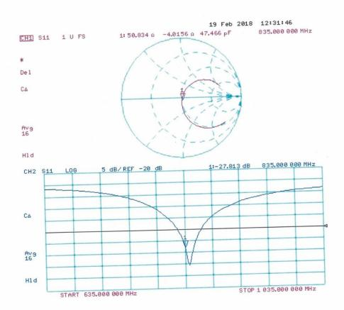
Impedance Measurement Plot for Head TSL
