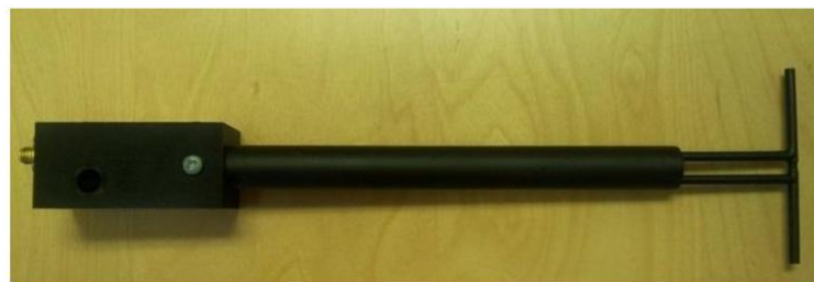
Figure 1 – MVG COMOSAR Validation Dipole
