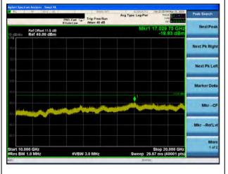
Conducted Emission Transmitting Mode CH 9538 10GHz – 20GHz
