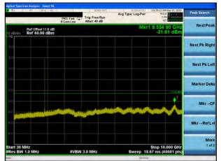
Conducted Emission Transmitting Mode CH 4233 5GHz – 10GHz
