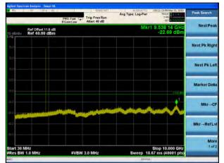
Conducted Emission Transmitting Mode CH 251 5GHz - 10GHz
