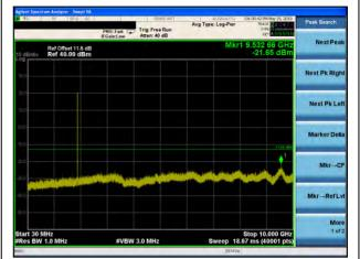
Conducted Emission Transmitting Mode CH 9400 10GHz – 20GHz
