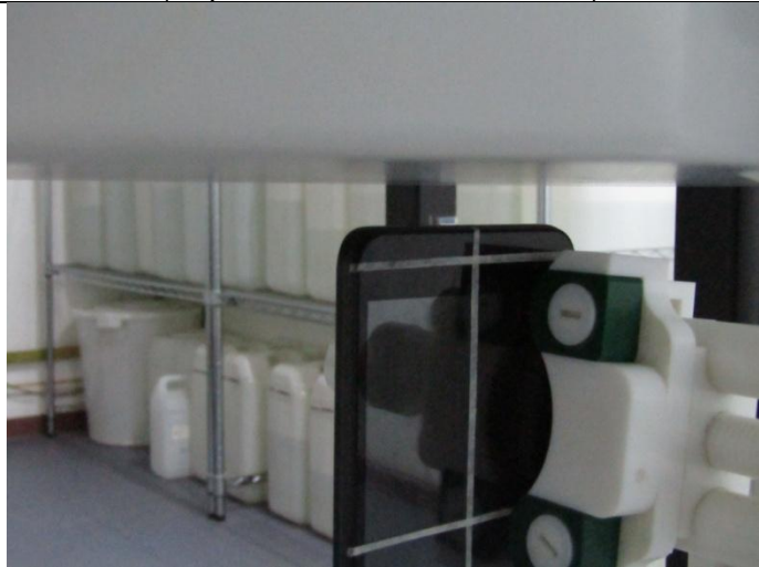
Top Side (Separation distance of 10mm)
