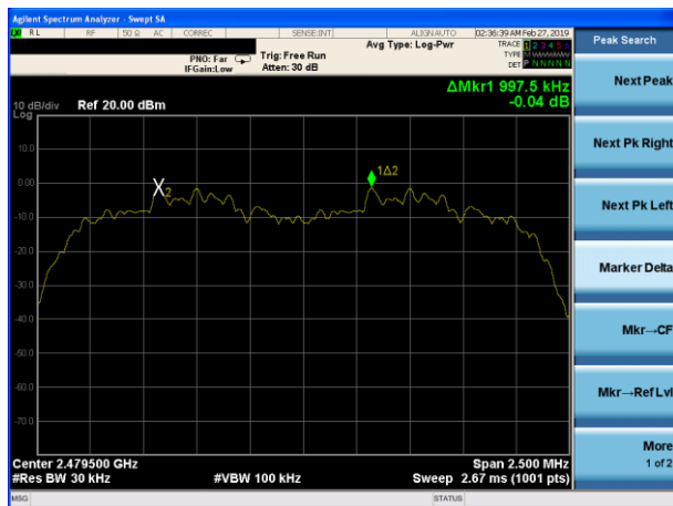
(3Mbps) Channel Separation plot on channel 77-78
