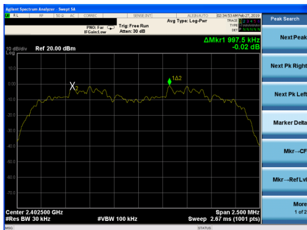
(3Mbps) Channel Separation plot on channel 00-01
