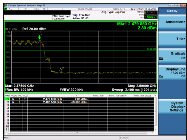
8-DPSK: Band Edge-High Channel (Hopping Mode)
