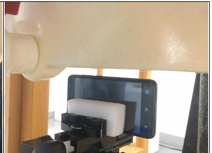
Right Side of EUT with 1.0 cm Gap
