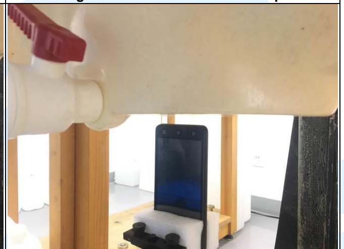
Bottom Side of EUT with 1.0 cm Gap
