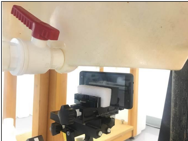
Left Side of EUT with 1.0 cm Gap
