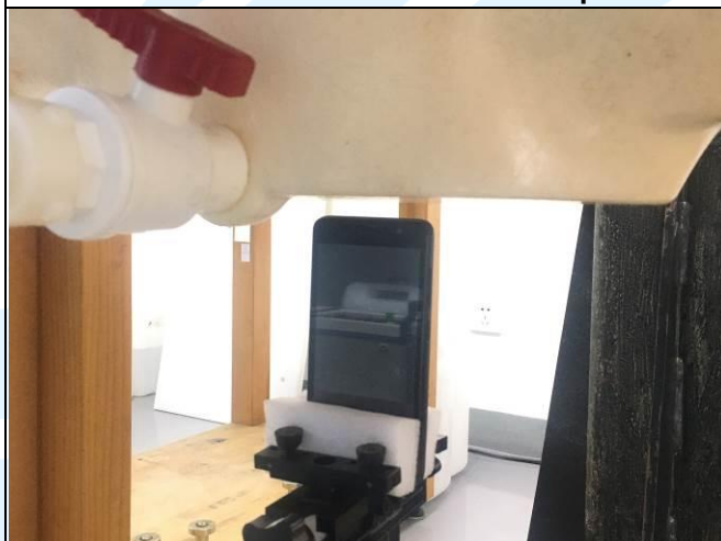
Top Side of EUT with 1.0 cm Gap
