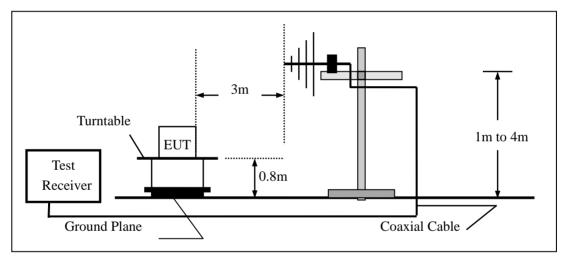
(c) For radiated emissions above 1000MHz
