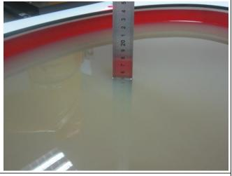
Liquid depth in the Body phantom
