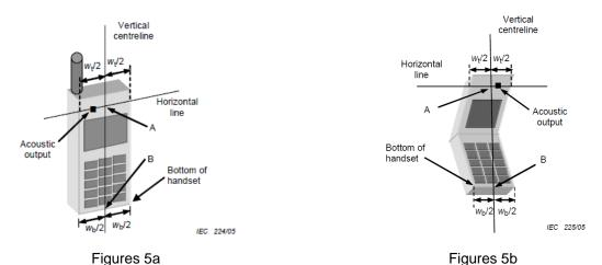
W<sub>t</sub> Width of the handset at the level of the acoustic
