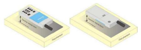
Picture 4 Test positions for body-worn devices
