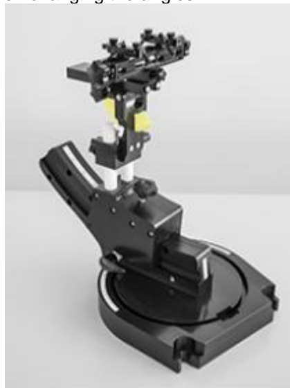
Device holder supplied by SPEAG
