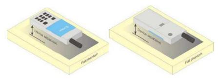
Picture 4 Test positions for body-worn devices
