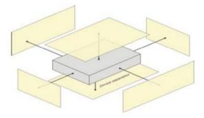
Picture 5 Test positions for Hotspot Mode
