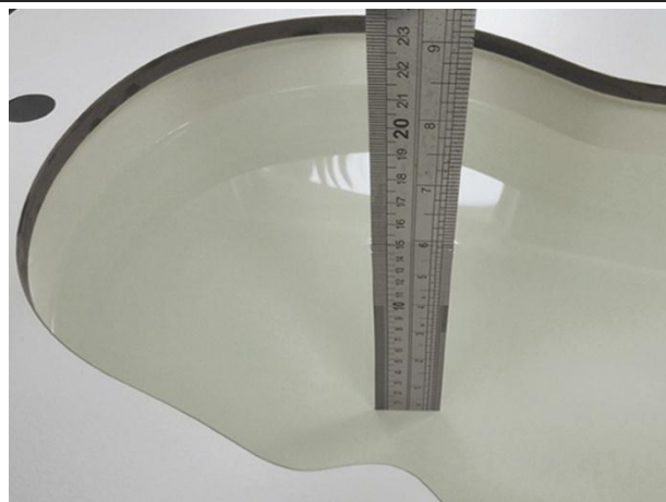
Liquid depth in the head phantom (2450MHz)
