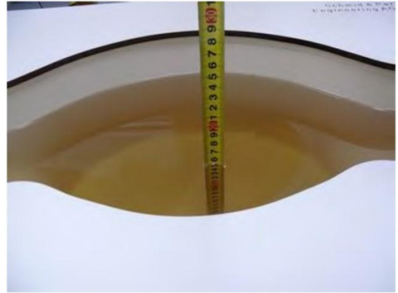
Liquid depth in the body phantom (835MHz)
