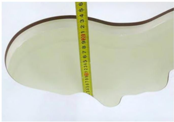
Liquid depth in the head phantom (1900MHz)
