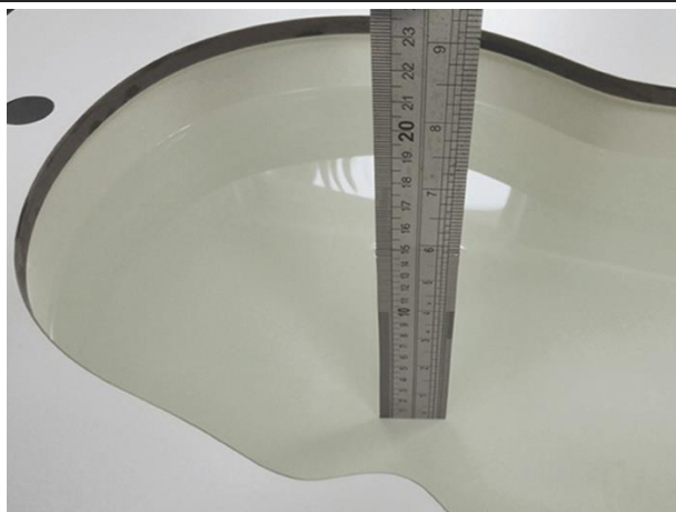
Liquid depth in the head phantom (2450MHz)
