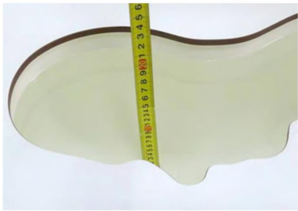
Liquid depth in the head phantom (1900MHz)
