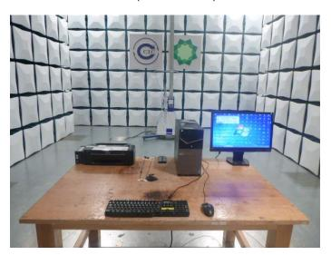
Radiated Emission (above 1GHz) Connect to PC
