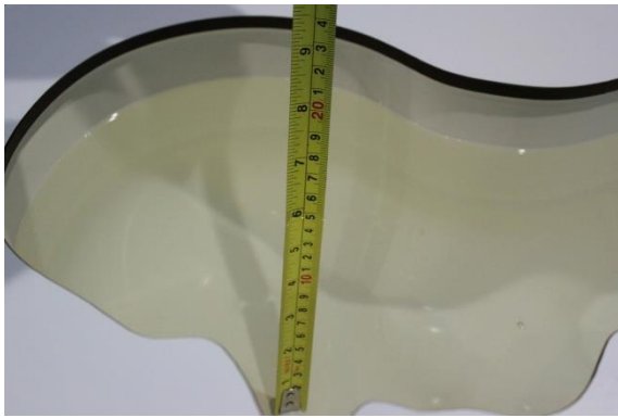
Liquid depth in the head phantom (2600MHz)
