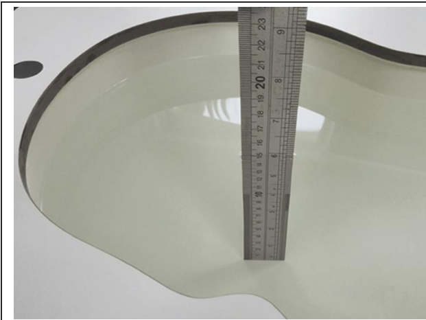
Liquid depth in the head phantom (2450MHz)
