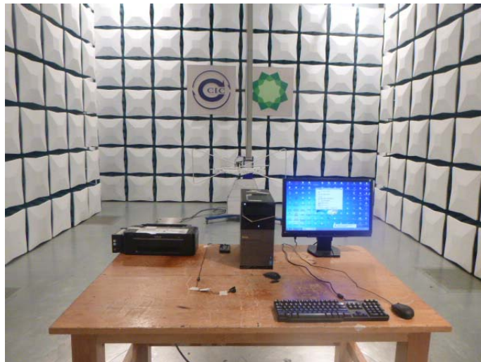
Radiated Emission (above 1GHz) Connect to PC
