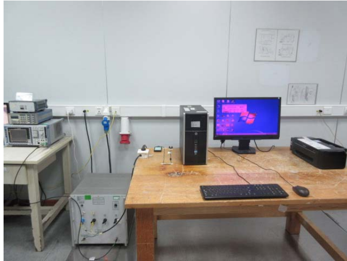
Radiated Emission (30MHz-1GHz) Connect to PC
