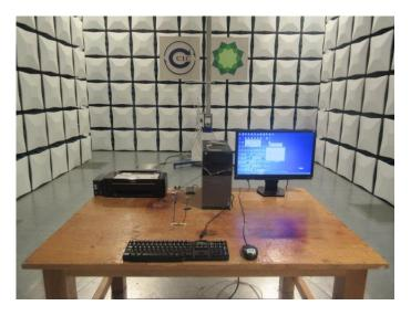
Radiated Emission (above 1GHz) Connect to PC
