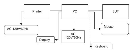
**Equipment Used in Tested System**
