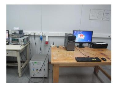
Radiated Emission (30MHz-1GHz) Connect to PC
