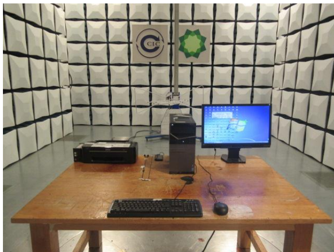
Radiated Emission (above 1GHz) Connect to PC
