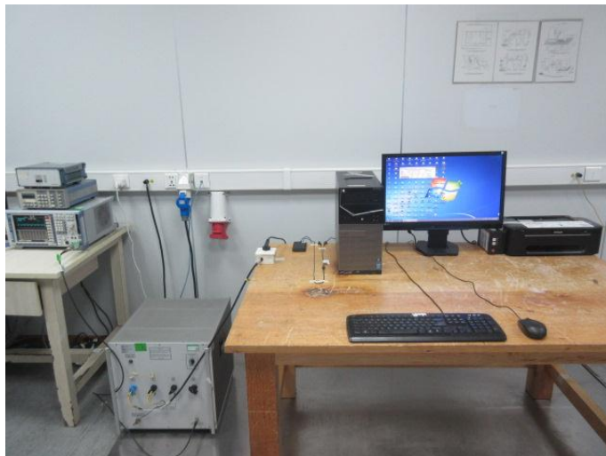
Radiated Emission (30MHz-1GHz) Connect to PC
