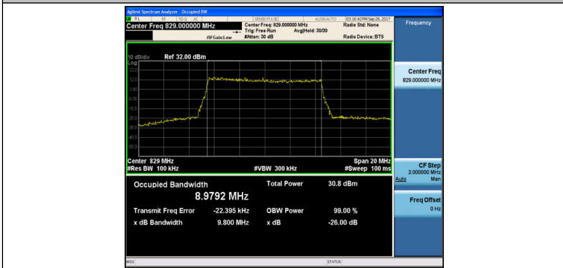
Band5_10MHz_16QAM_20450_50RB#0_8.9643_9.799_PASS
