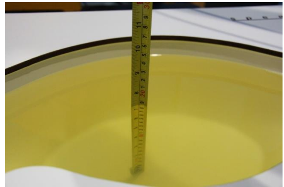
Liquid depth in the body phantom (1750MHz)
