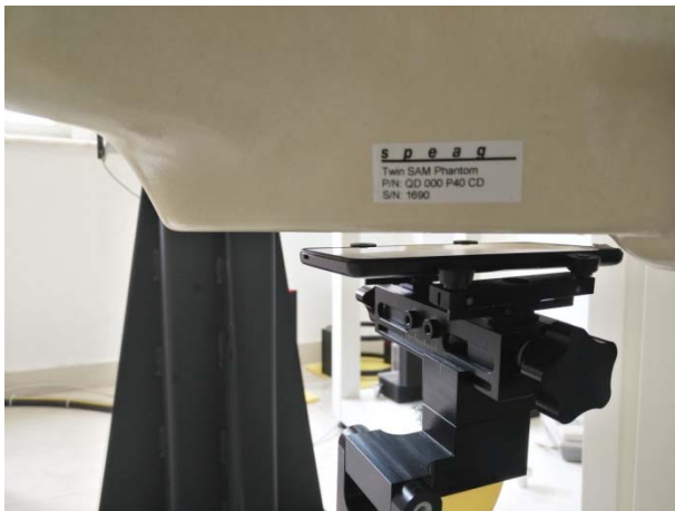
Body-worn Front Side (10mm)
