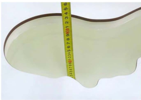
Liquid depth in the head phantom (835MHz)
