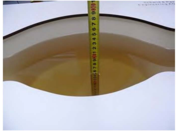
Liquid depth in the body phantom (835MHz)
