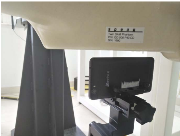
Hotspot mode - Left Side (10mm)
