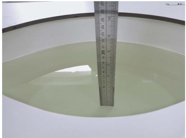
Liquid depth in the body phantom (2450MHz)
