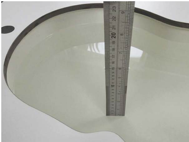
Liquid depth in the head phantom (2450MHz)
