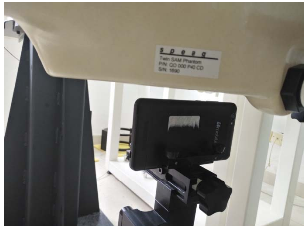
Hotspot mode - Right Side (10mm)
