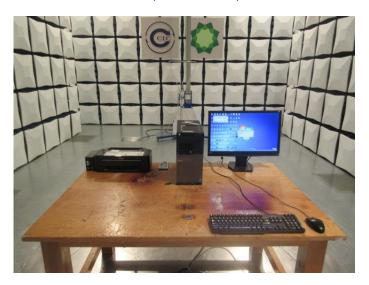
Radiated Emission (above 1GHz) Connect to PC
