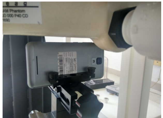
Hotspot mode - Right Side (10mm)
