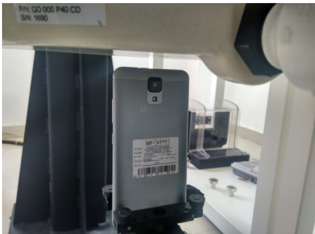
Hotspot mode - Top Side (10mm)
