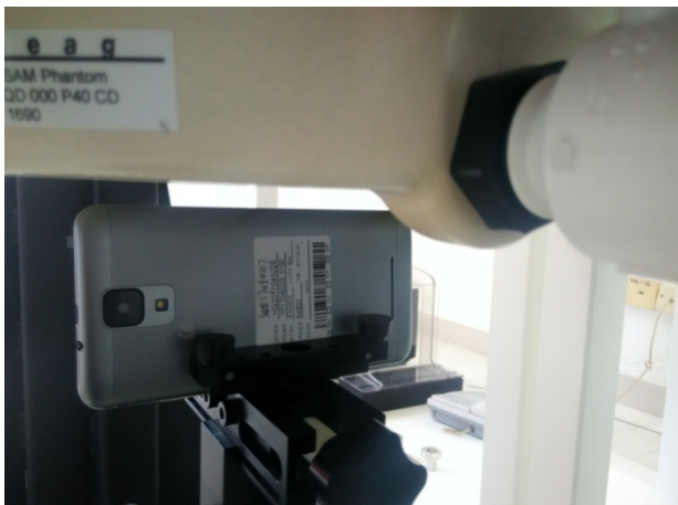
Hotspot mode - Left Side (10mm)
