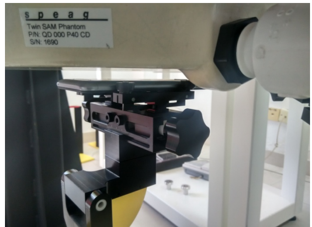
Body-worn Rear Side (10mm)
