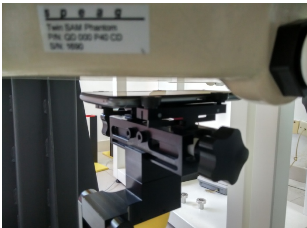
Body-worn Front Side (10mm)
