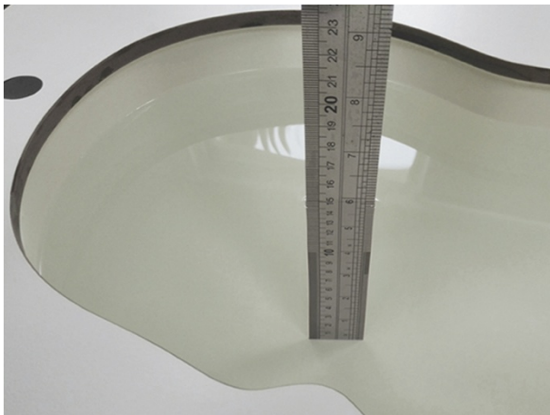
Liquid depth in the head phantom (2450MHz)
