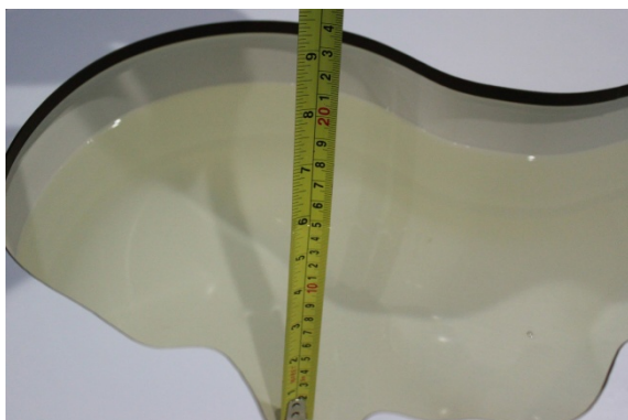
Liquid depth in the head phantom (2600MHz)
