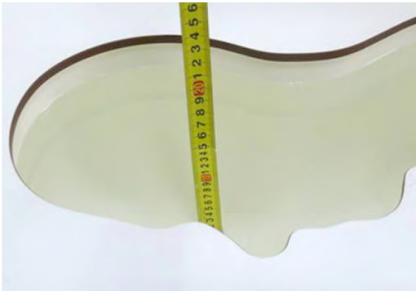
Liquid depth in the head phantom (835MHz)
