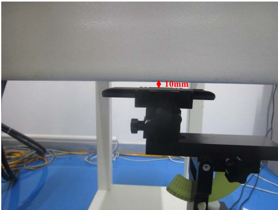
Body Back Setup Photo(10mm)
