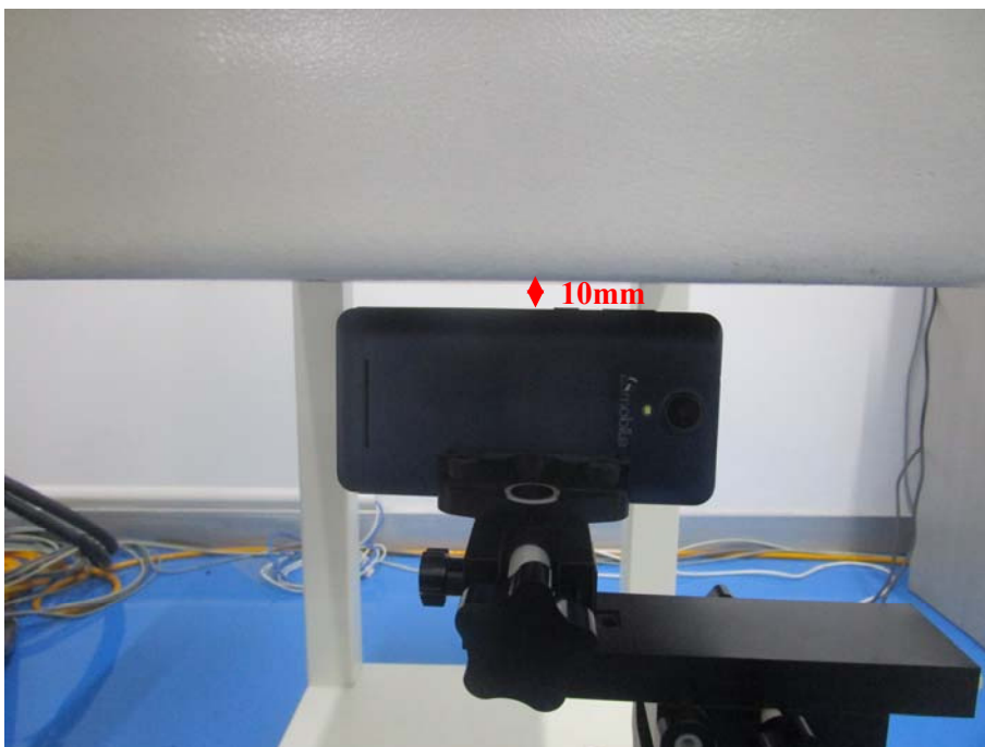
Body Right Setup Photo(10mm)
