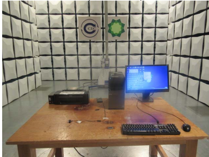
Radiated Emission (above 1GHz) Connect to PC
