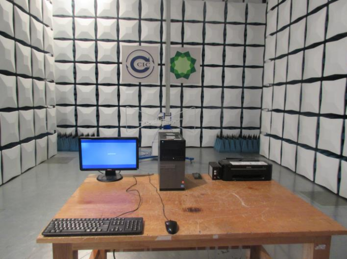
Radiated Emission (above 1GHz) Connect to PC
