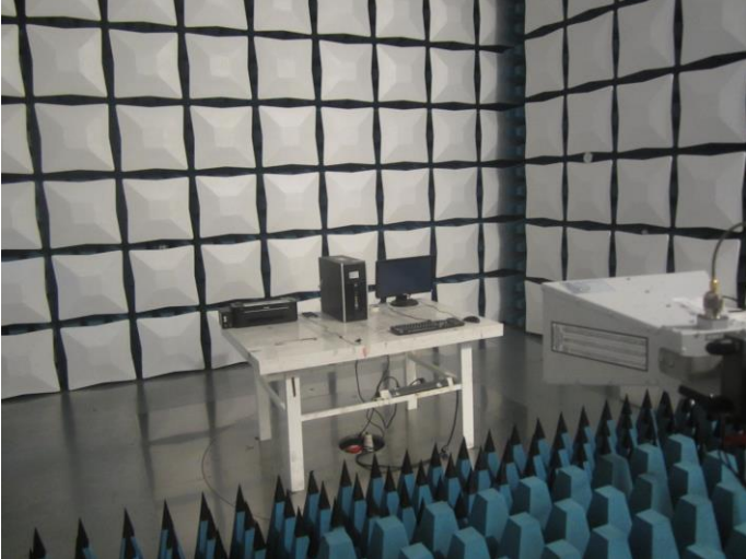
Radiated Emission (above 1GHz) Connect to PC
