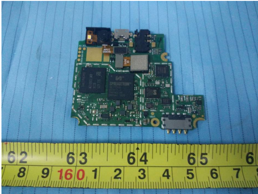
EUT – Mainboard Top Shielding off View
