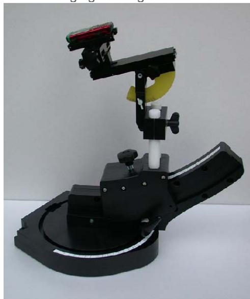
Device holder supplied by SPEAG
