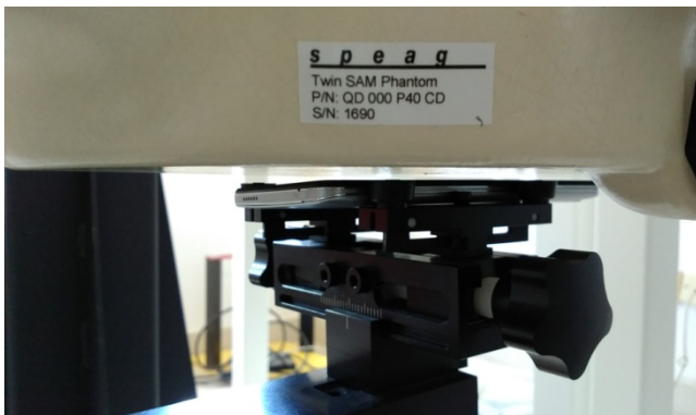
Body-worn Front Side (5mm)
