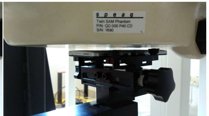
Body-worn Rear Side (5mm)
