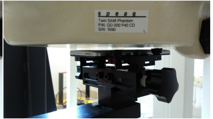
Hotspot mode - Rear Side (10mm)
