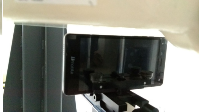
Hotspot mode - Right Side (10mm)
