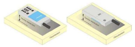
Picture 4 Test positions for body-worn devices
