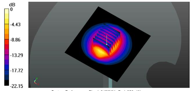
System Performance Check 2450MHz Body250mW
