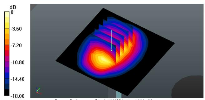
System Performance Check 1900MHz Head 250mW
