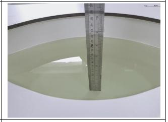
Liquid depth in the head phantom (2450MHz)
