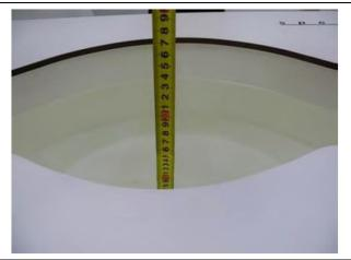
Liquid depth in the head phantom (1900MHz)
