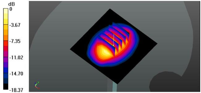
System Performance Check 1900MHz Body250mW
