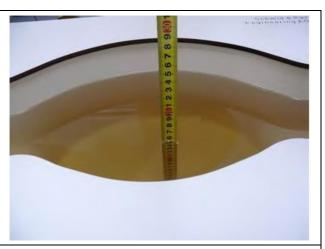
Liquid depth in the body phantom (835MHz)
