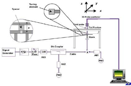
The output power on dipole port must be calibrated to 24 dBm (250mW) before dipole is connected.
