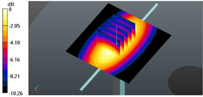
System Performance Check 835MHz Body 250mW
