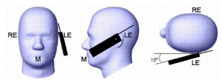
Picture 3 Tilt position of the wireless device on the left side of SAM
