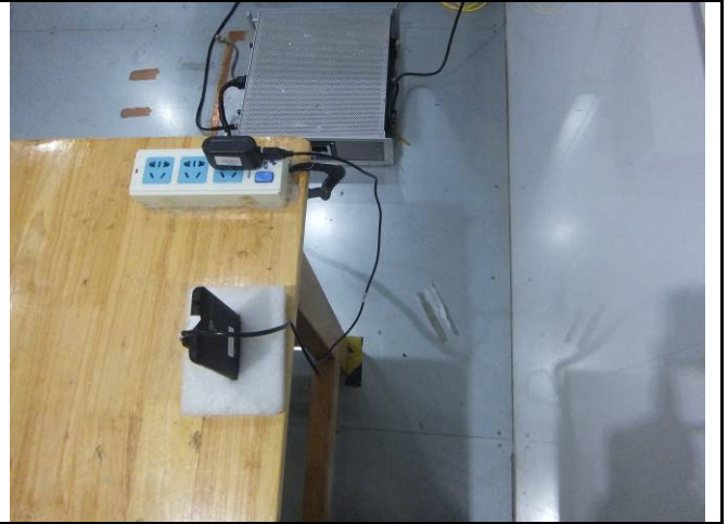
Conducted Emissions Test Setup Side View
