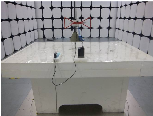
Conducted Emissions Test Setup Front View
