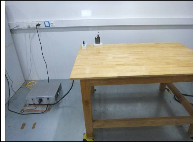
Conducted Emissions Test Setup Front View
