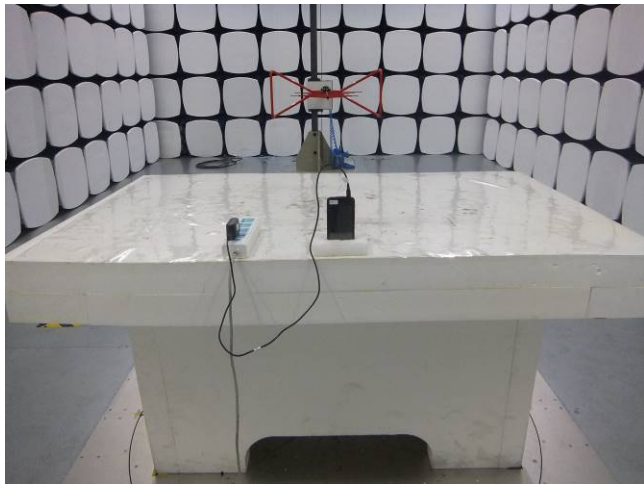
Conducted Emissions Test Setup Front View
