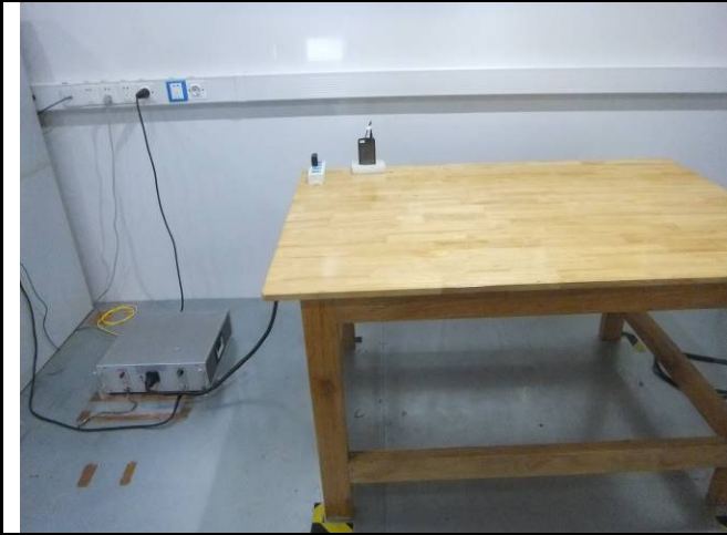
Conducted Emissions Test Setup Front View
