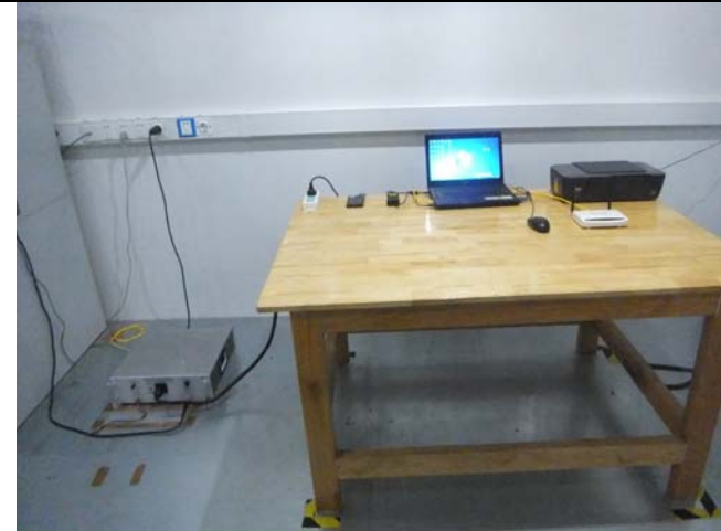
Conducted Emissions Test Setup – Front View
