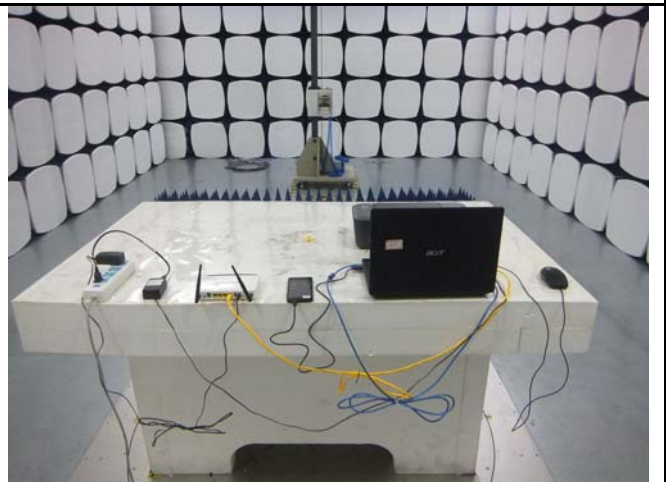
Radiated Spurious Emissions Test Setup Above 1GHz
