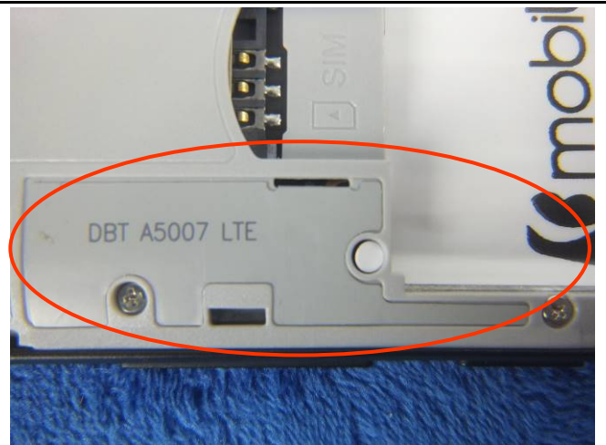
LTE- Antenna View
