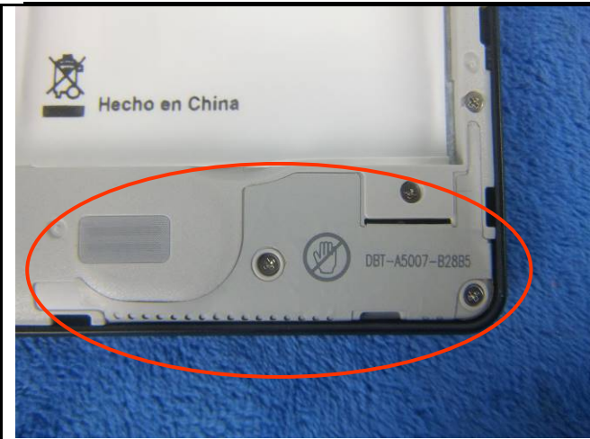
GSM/PCS/UMTS-FDD Antenna View
