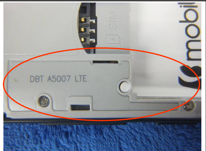
LTE- Antenna View
