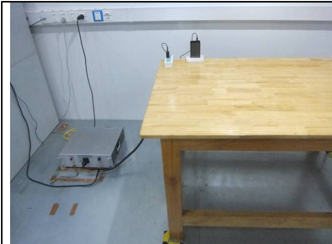
Conducted Emissions Test Setup Front View
