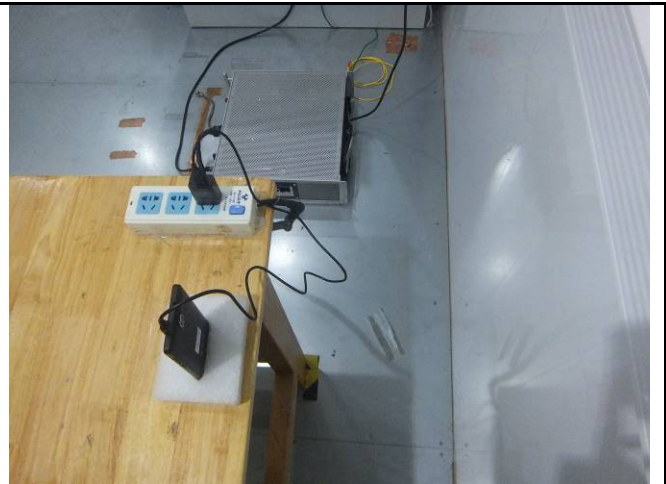
Conducted Emissions Test Setup Side View
