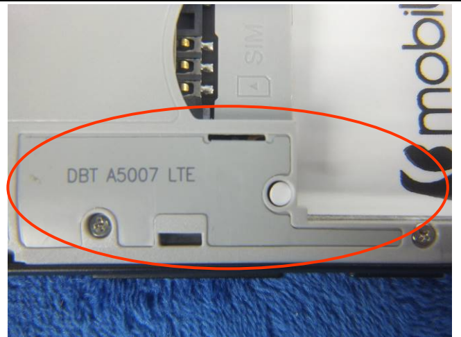
LTE- Antenna View
