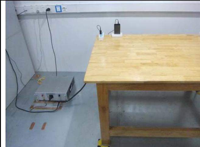
Conducted Emissions Test Setup Front View
