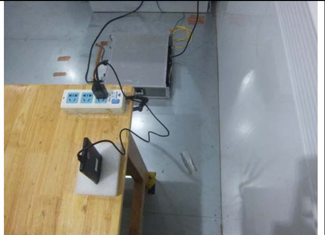
Conducted Emissions Test Setup Side View
