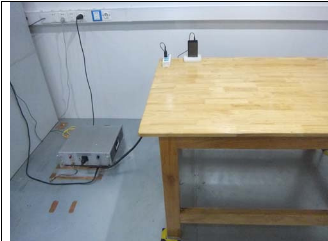
Conducted Emissions Test Setup Front View
