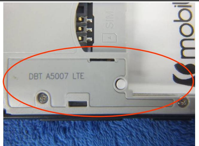
LTE- Antenna View
