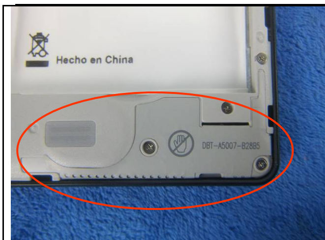
GSM/PCS/UMTS-FDD Antenna View
