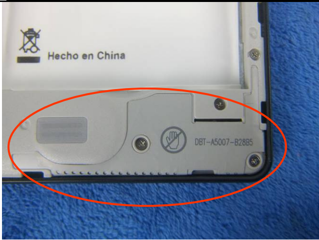
GSM/PCS/UMTS-FDD Antenna View
