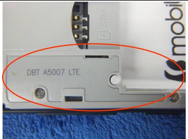
LTE- Antenna View
