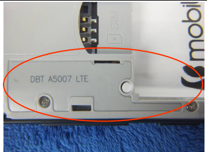
LTE- Antenna View
