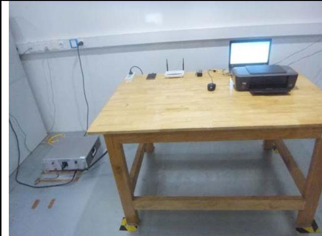
Conducted Emissions Test Setup – Front View
