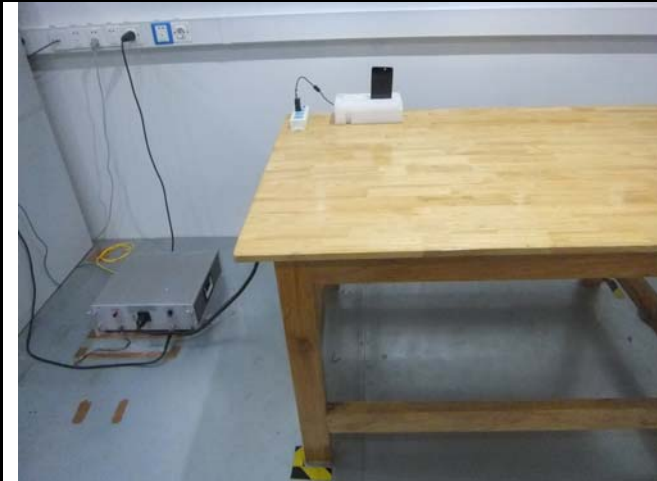
Conducted Emissions Test Setup Front View
