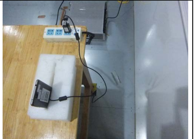
Conducted Emissions Test Setup Side View
