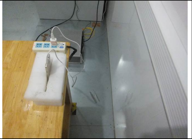
Conducted Emissions Test Setup Side View
