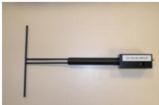
Figure 1 – Satimo COMOSAR Validation Dipole
