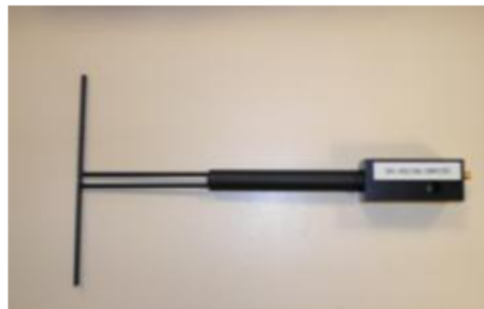
Figure 1 – Satimo COMOSAR Validation Dipole
