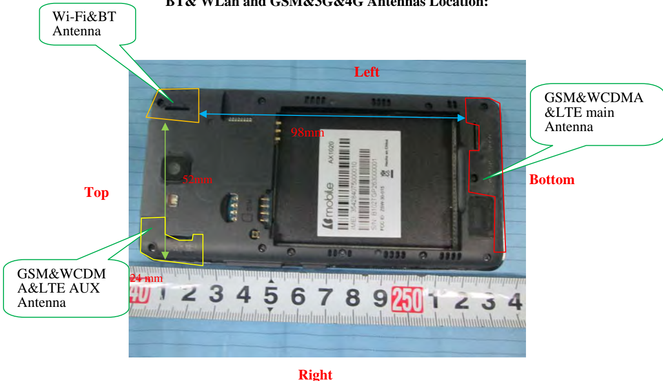
BT& Wlan and GSM&3G&4G Antennas Location:
