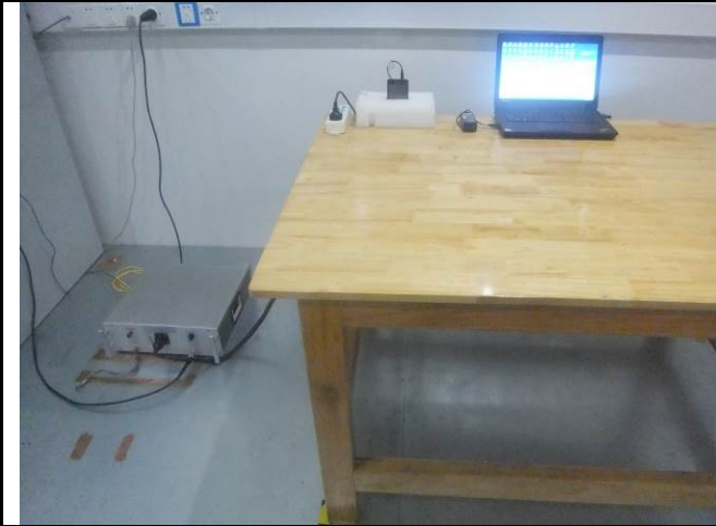
Conducted Emissions Test Setup – Front View
