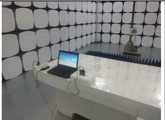
Radiated Spurious Emissions Test Setup Above 1GHz
